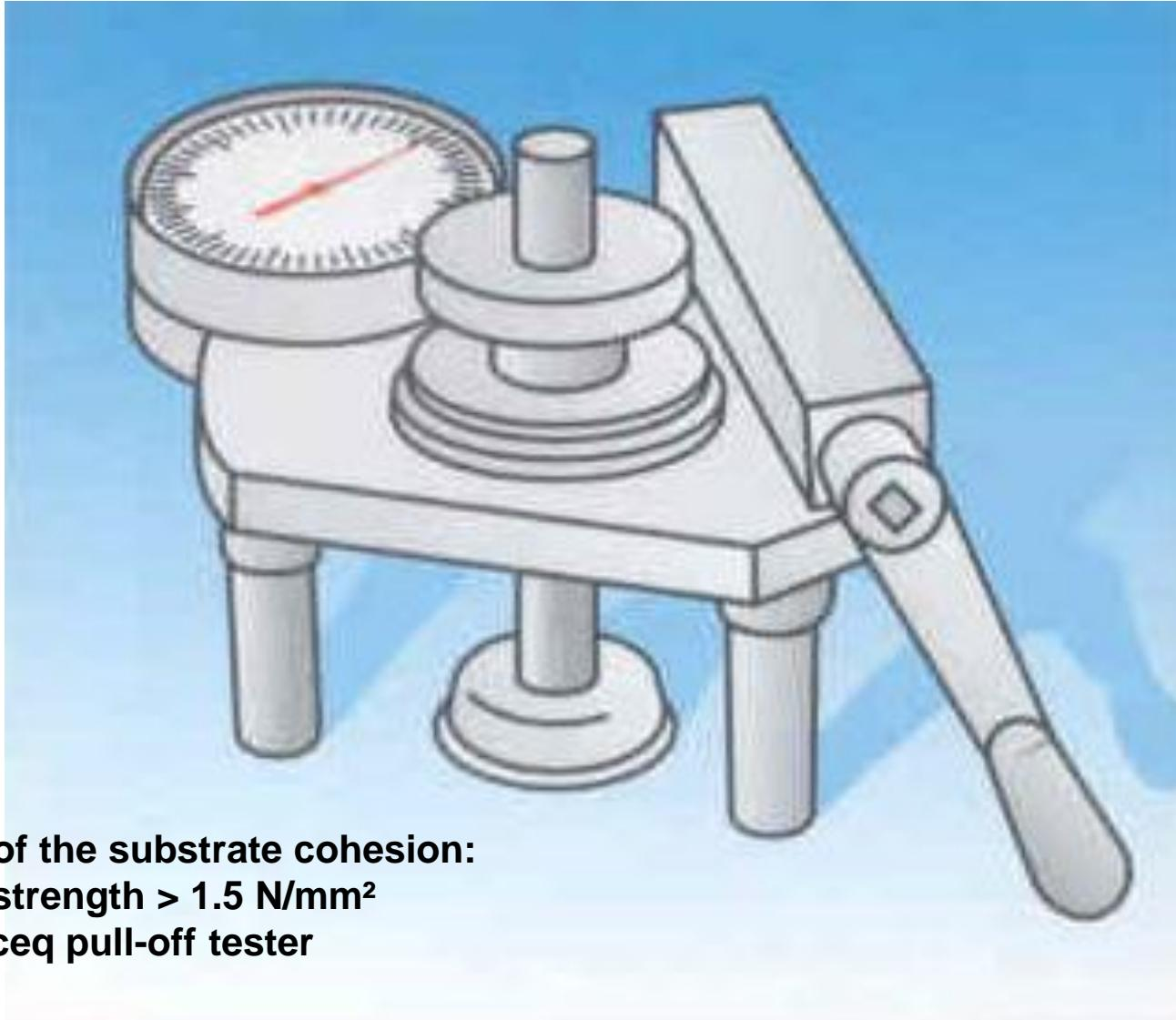
Testing of the substrate cohesion:
