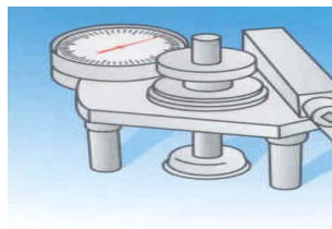
Testing of the substrate Pull-off strength > 1.5 N/mm 2 . E.g. Proceq, Dyna pull-off tester.
